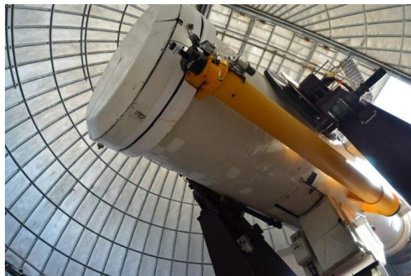
Figure 2: TESCA, the Calern observatory Schmidt telescope. (© OCA).
