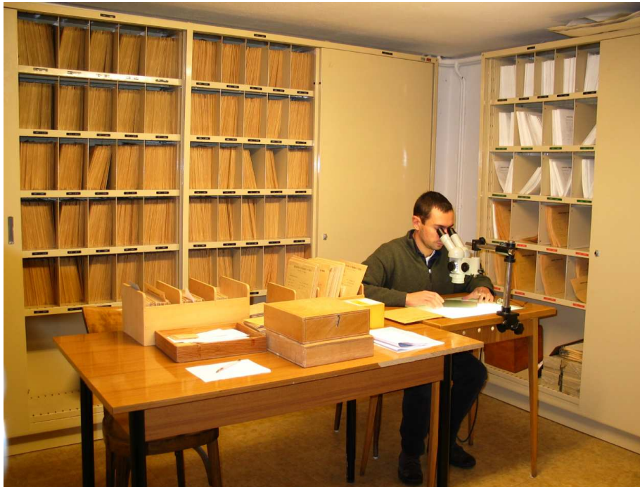
Figure 3: The Asiago plate archive. The temperature is stable through the year and the humidity is controlled. Plates are store vertically in soft, non-abrasive paper envelopes. Three binocular Zeiss microscopes and two large area flat-bed scanners are available to assist.
